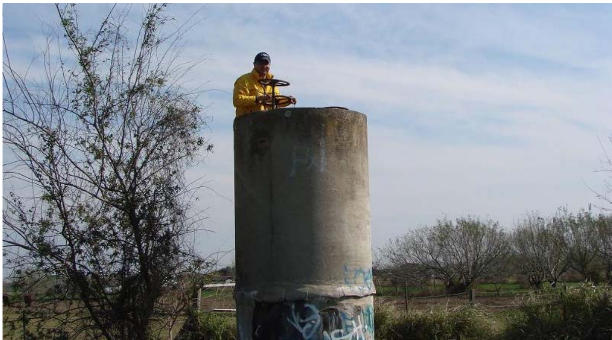
Figure 8. Askar Karimov, Extension Associate, is shown taking the measurement from the top inside rim of a standpipe.
