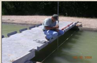
Askar measures the maximum flow of the old control structure with a propeller meter
