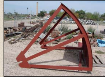
The new Radial gate was delivered
