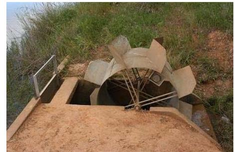
Australians use a unique water wheel system for measuring on-farm flow.
