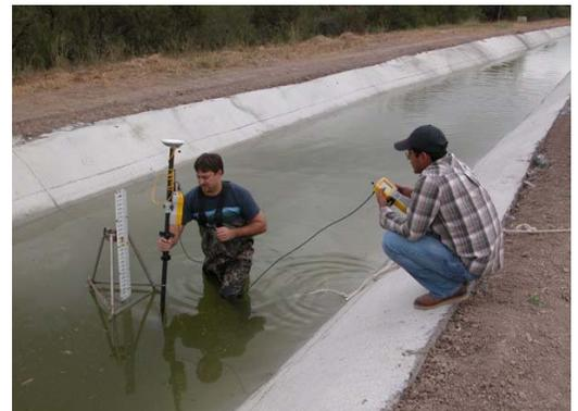
GPS surveying of the canal cross section and the staff gauge.
