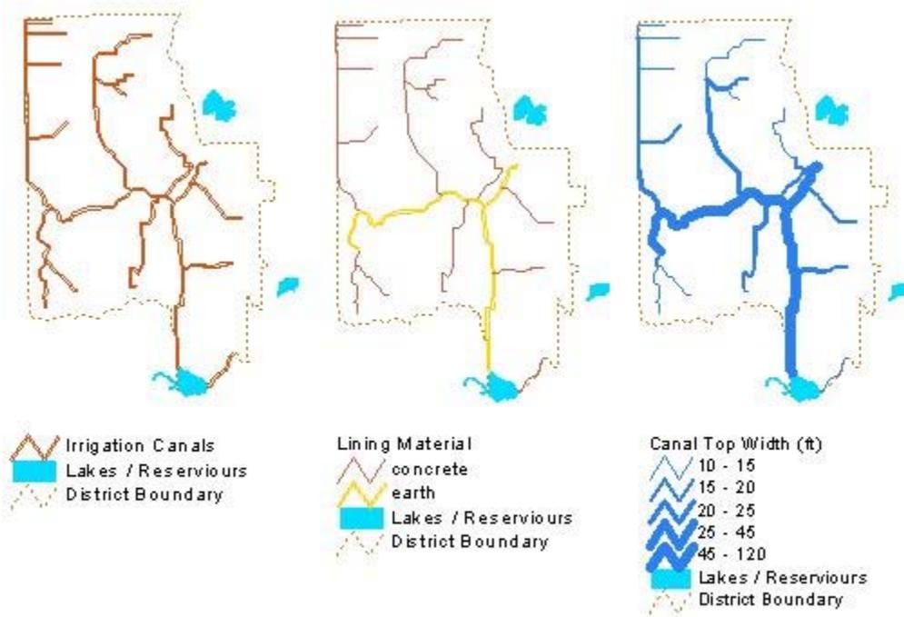
Figure 3. The main distribution system of the Mercedes Irrigation District and various ways of displaying its attributes for analysis, including the lining classification and canal size.
