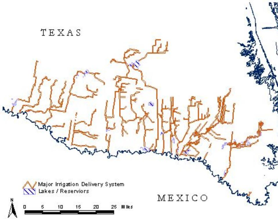
Figure 4. Main irrigation distribution systems in the Lower Rio Grande Valley.
