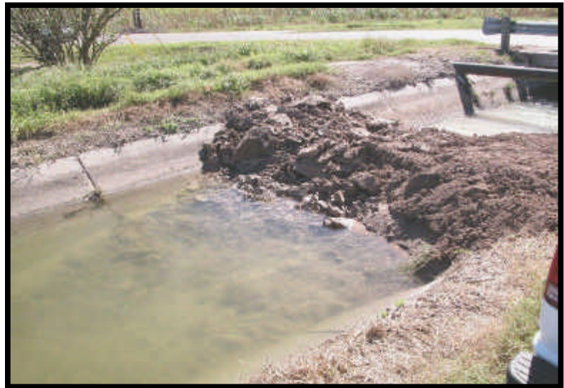
Figure A3. Close up of an earthen dam used in ponding tests.
