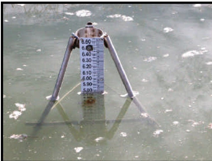
Figure A4. Free standing staff gauge used to record changes in water levels during test.
